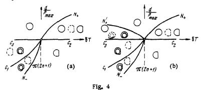
of parameter variation satisfying condition (3, 12) we expect a hard doubling of the oscillation period (Fig. 4b). Quite naturally, a structure of decomposition of the parameter space into domains of periodic motions of various types more complicated than that in Fig. 4 is possible in the neighborhood of bifurcation nodes.
